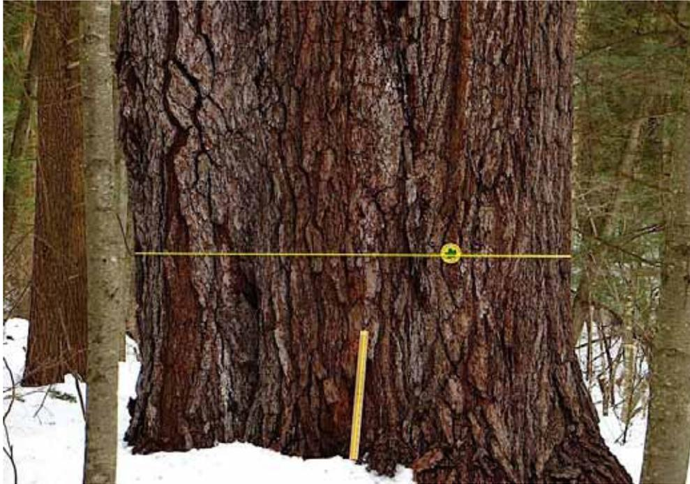
In the photograph, the object of known size, called the reference object, is an 18-inch ruler. It is oriented close to 90 degrees to the line of sight. The diameter of the trunk is also oriented 90 degrees to the line of sight.
