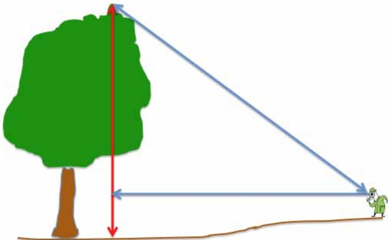
In the diagram, the horizontal blue line is the true baseline. It does not extend all the way to the trunk.
