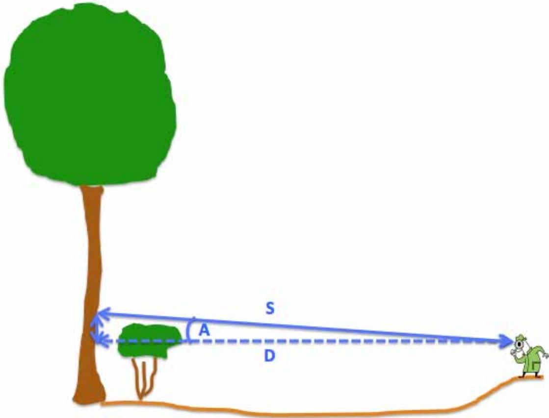
Shoot to a convenient point on the trunk with a laser (or possibly measure with a tape), take the vertical angle to that point, and apply the following formula:
