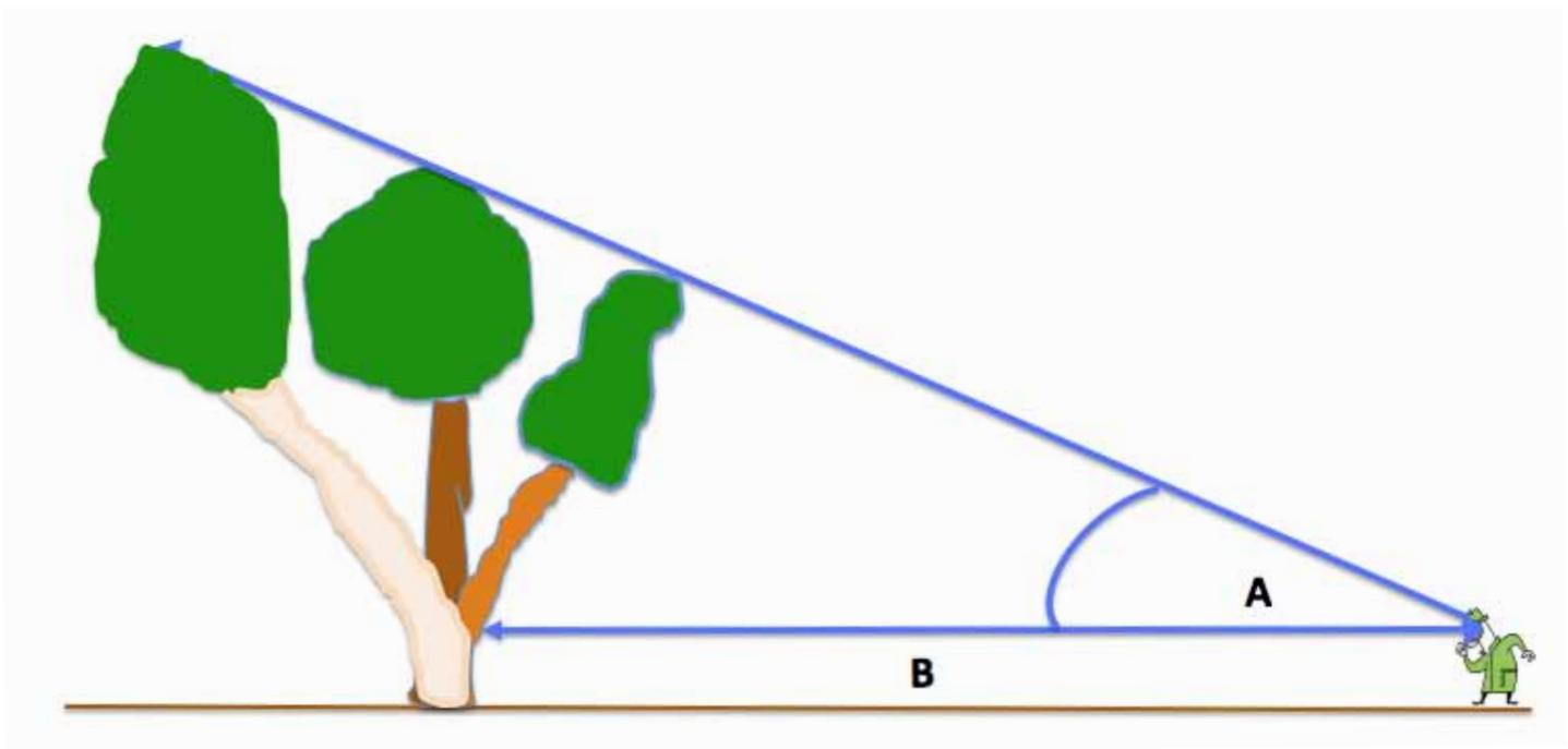
The measurer should try to find the spot on the ground directly beneath the top. The horizontal distance from the eye to this spot is the correct baseline for the top. Even approximating this distance is better than generating a large error in height from using an incorrect baseline. The diagram below illustrates this technique.
