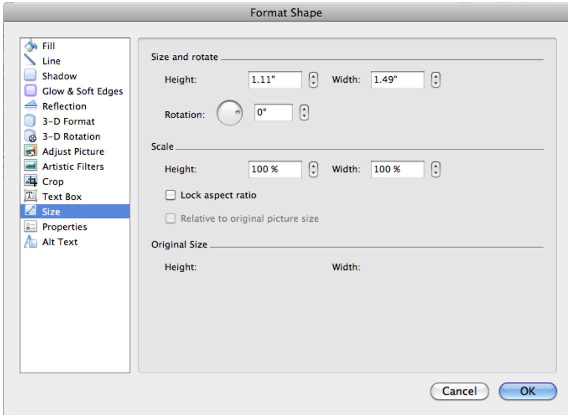
d. The size for a line is presented in Excel as the dimensions of a rectangle. The line becomes its diagonal. In the above example, the height of the box is 1.11 units and the width is 1.49. The actual size of the line, meaning its length, is the diagonal of the rectangle with those dimensions.
