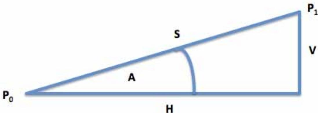
In the above diagram, three distances can be associated with the line  $P_0P_1$ . The linear path  $S$  is often called the slope distance. The vertical separation between  $P_0$  and  $P_1$  is defined as  $V$  and the horizontal separation is defined as  $H$ . The vertical angle of  $P_1$  relative to  $P_0$  is defined as  $A$ . The triangle  $SVH$  is a right triangle by virtue of the fact that  $H$  and  $V$  are at a right angle to one another.
