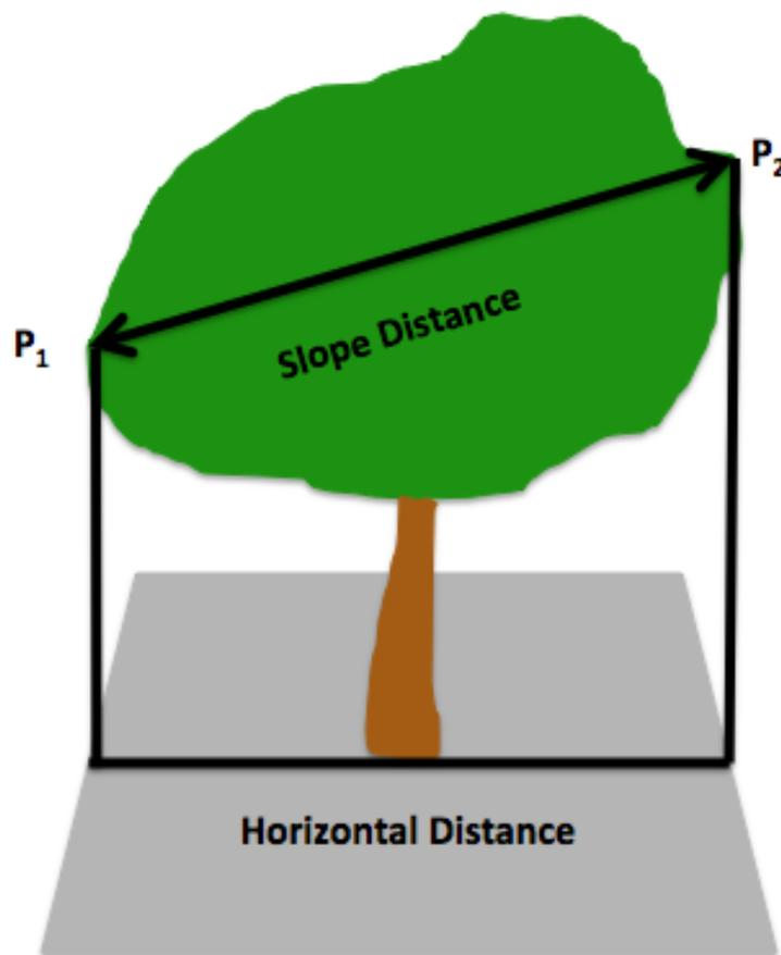
When you cannot position yourself under the crown, you must use our third approach, which measures crown spread from a distance. This method makes use of the vertical plane as seen from the side, a camera's eye view, shown below.
