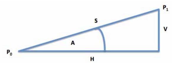
**Diagram of Distance Components Between Two Points**
