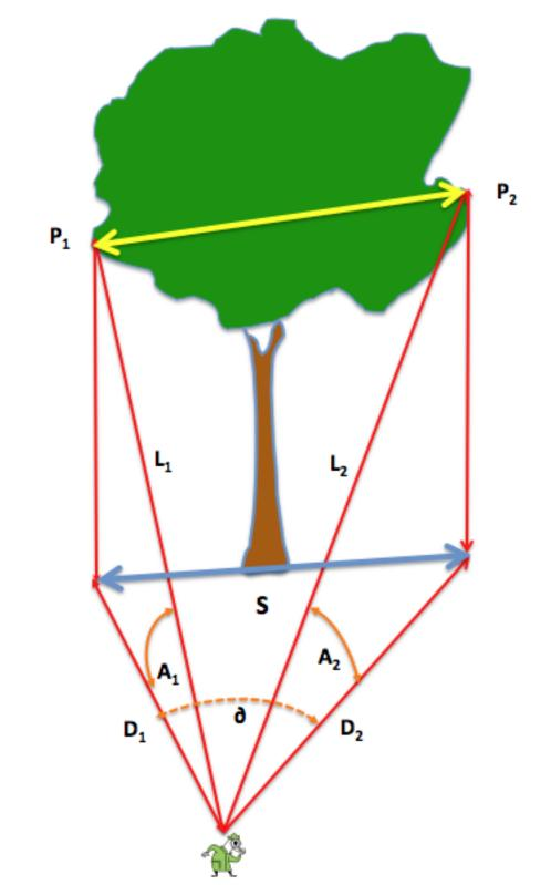
**Diagram of Azimuth Difference Crown-Spread Method**
