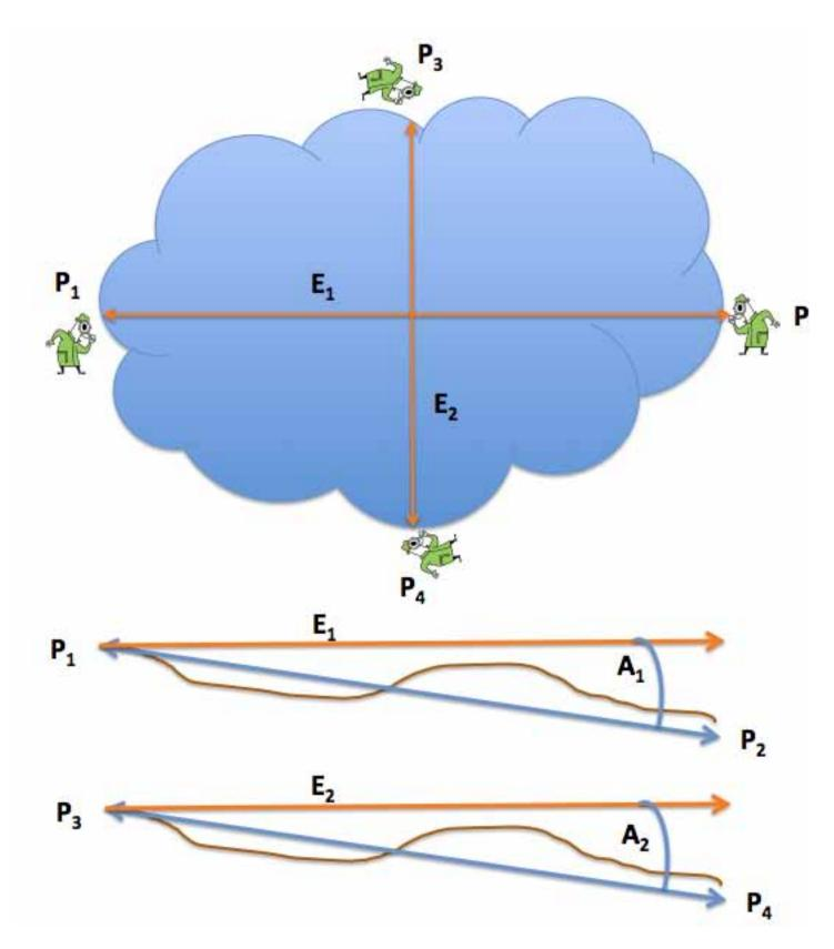
The lower part of this diagram illustrates that the paths from  $P_1$  to  $P_2$  and  $P_3$  to  $P_4$  are slope distances. The orange lines are the horizontal distances we seek.
